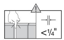
CAUTION: Spacing between boards must be less than 1/4" or a finger entrapment could exist.
