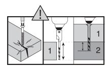
CAUTION: These boards should be pre-drilled and countersunk to avoid cracking. *Note: Adjust countersink tool to width of first board to countersink to proper depth. Pre-drill into second board using first board as a template before attaching.*
