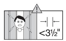
CAUTION: Spacing between boards must be less than 31/2" (or greater than 9") or a head/neck entrapment could exist.
