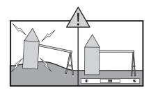
CAUTION: Ground must be level. Installation on a hill or incline will create unsafe conditions.
